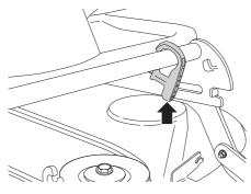
5 Lift off the drive belt and hang on the load-relieving hook.
